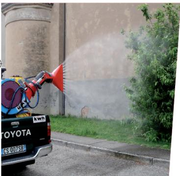
The perfect and **uniform micronization** produced using a unique type of pneumatic nozzle, with a large diameter (4 mm), and **fade-free functionality, no wear**, no clogging, no maintenance.
